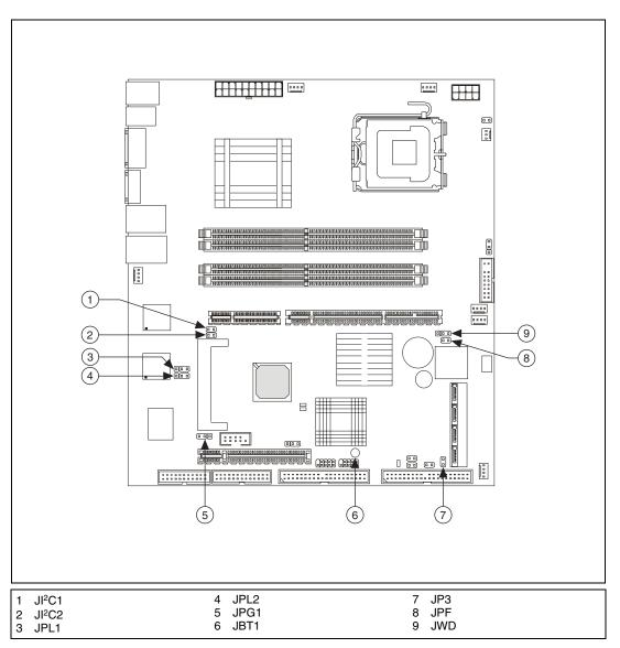
Figure B-2 shows the jumper locations on the NI 8352/8353.
